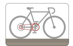
A cyclist can ride up a hill by using a small gear that is easier to pedal attached to a larger gear, which turns the back wheel slowly but with more force.
