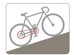
Using gears of the same size with the same number of teeth does not give a mechanical advantage because both gears turn with the same force and at the same speed.
